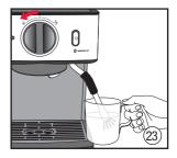
Place steam wand into milk, approx. 1cm below surface and turn the dial to the steam  $\boldsymbol{b}$  setting.
